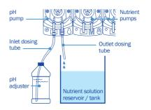
To set up nutrient tubing and pumps, repeat steps 1-4 using the darker nutrient solution tubing. For the L Version: Insert and twist each connector of the nutrient dosing tube into each nutrient pump tube connector.
