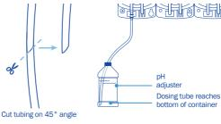
3 Set up the outlet dosing tube. M Version: use the remaining dosing tube with the connector, and insert the connector into the RIGHT pH pump tube.
