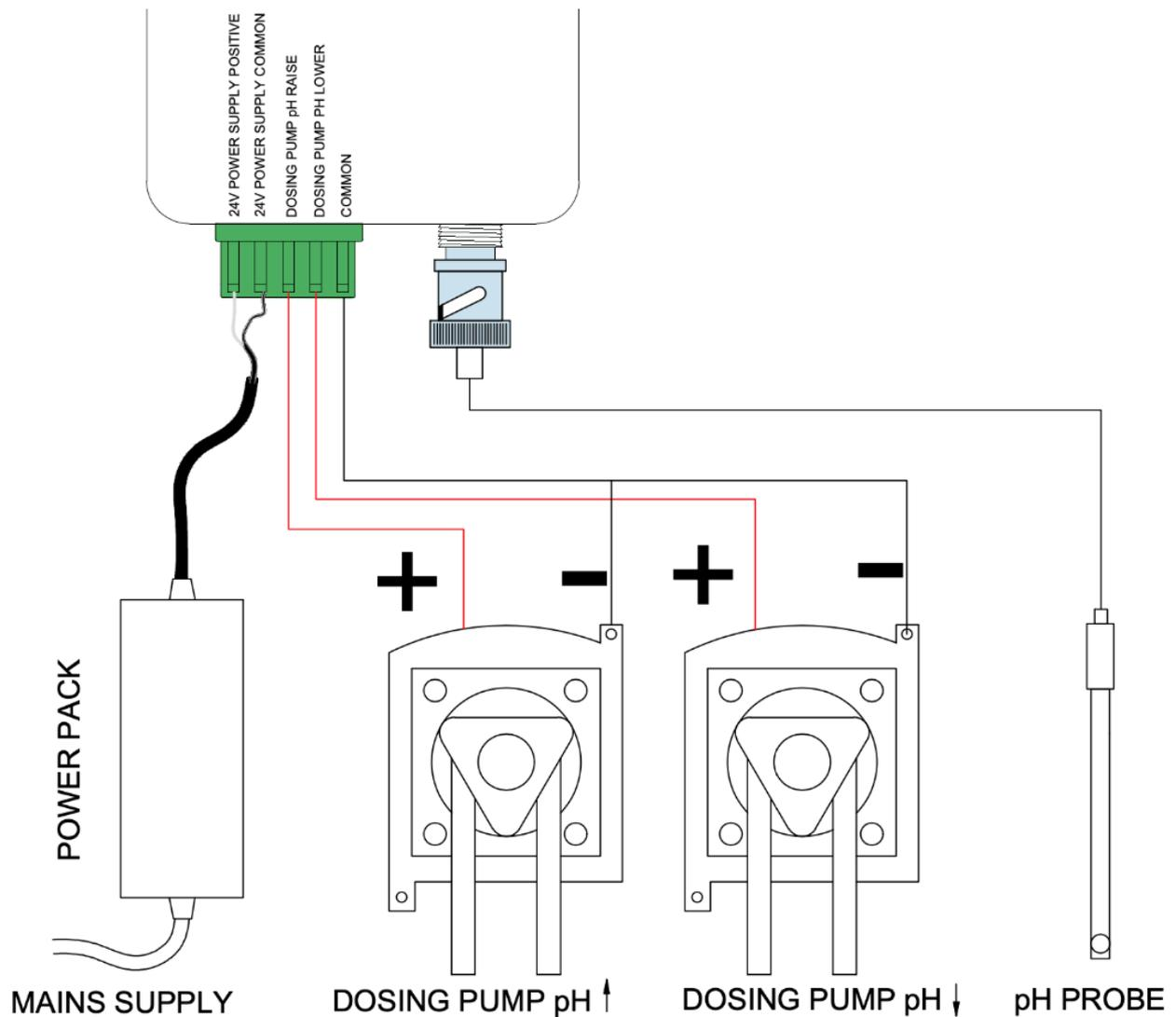
Note: that all the connections marked **24V Common** are connected internally and you may connect the return wire from any pump to any of these commons. The 24V live wire is normally marked by a white stripe or white printing along its length.
