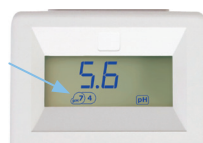
Successful pH 7 and pH 4 calibration
